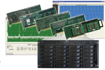
Create a synchronized multi-channel acquisition recording system with linked digitizers; acquiring and transfering data simultaneously to disc storage in real-time with no loss in data
